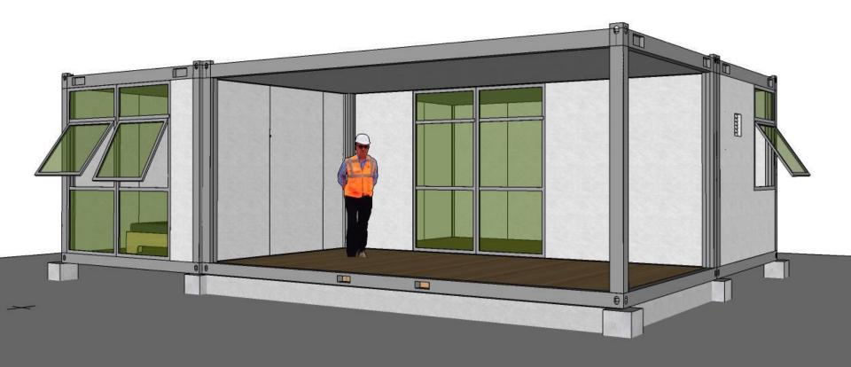
Design drawing is provided by client. The preliminary design is made in accordance to client' s requirement and local building code. After getting the permission by local authority, PTH will do the shop drawing for production.
